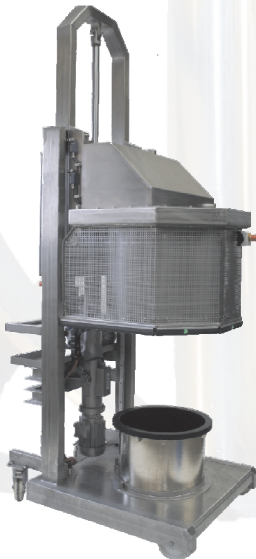
B 30 vacuum mixer mixing head lifted up
