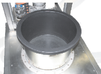
Container in stainless steel, teflon coats
